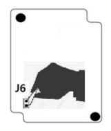
X Locate sensor powered at fresh air where Co gas is not exist (0ppm). Let J6's two holes short, using tweezers or so, to initiate Zero-calibration takes 2~2.5 minutes until LED blinking stop.
