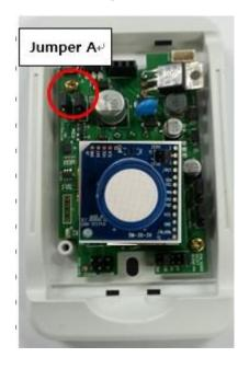
$4 \sim 20$ mA is default (2 ~ 10VDC or 0 ~ 20mA or 0 ~ 10VDC is selectable with jumper setting change)
