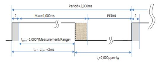
EX) t<sub>H</sub>(High Pulse Width) calculation for 400ppm in 2,000 ppm Range.
