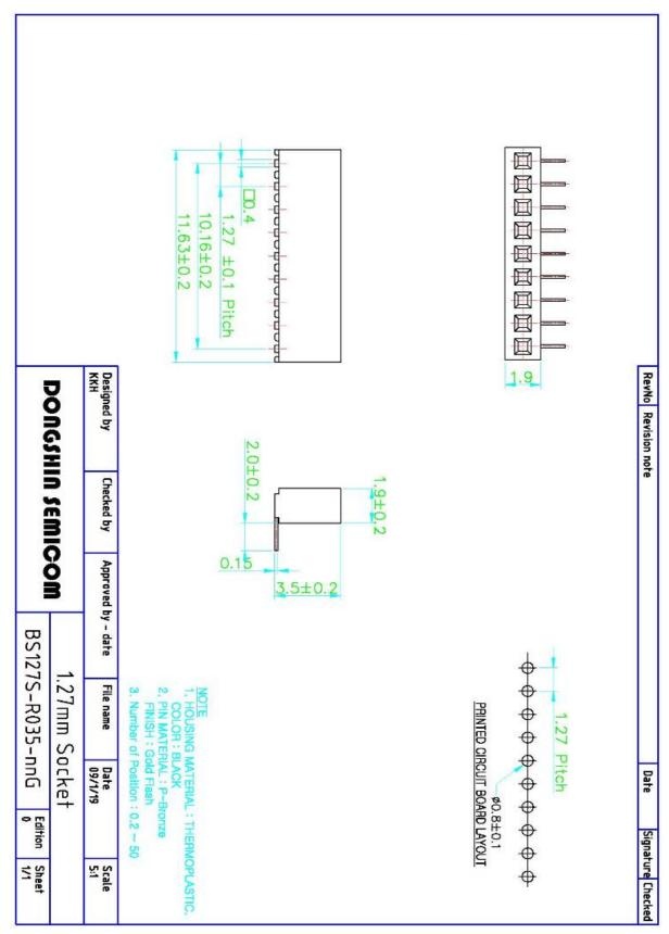
And 1.27mm center pin header recommended for mating with Socket of T-200.
